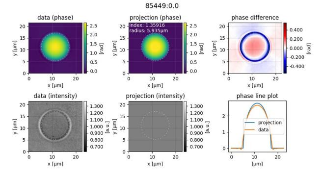
Note that the modeled intensity image is all-one, because the projection model only models the optical thickness and thus only affects the phase data. Also, note that the phase-difference image between data and model only has small deviations in the background phase. If there were large ramp-like structures or offsets, we would have to modify the *background correction*.
